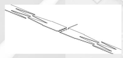
Hinge part is produced in one 150 mm width plate (except AT5 – 100 mm) and cut to the belt width. ERO Joint® HP belts are available with all types of coating and all types of guiding or machining.
