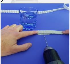
Begin to thread the pin by using an electric screwdriver and water (used as lubricant), to help the threading. For a correct alignment, use the plate/piece of belt furnished, like photo.
