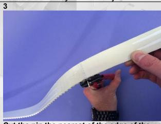
Cut the pin the nearest of the edge of the belt.
