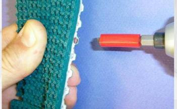
At the end of screwing, the tube slips on the tip to release the head of screw. Take care that the head of screw does not exceed the belt so that the screw does not rub on the pulleys.
