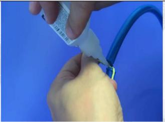
Eventually add a point of speed glue to seal it. Then make a second knot in the opposite direction of the previous knot (see sketch).
