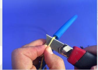
Cut the dangle strands (in case the welding of the belt is necessary, continue reading).
