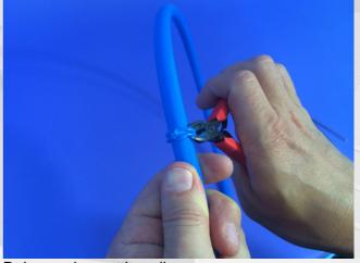
Deburr using cutting pliers.
